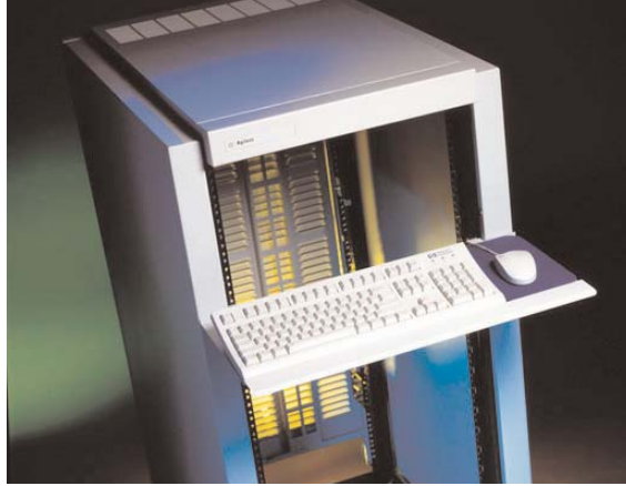
Fixed keyboard kit installed in rack
